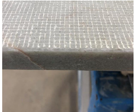
This is the underside of a slab, where the mesh goes all the way to the edge
