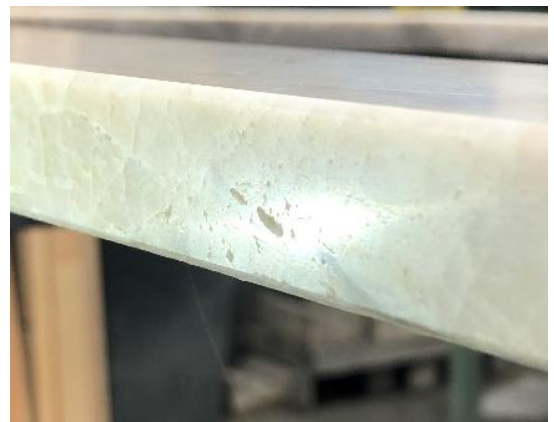
Small indentations often appear in the material on polished leading edges. These can also be felt.
