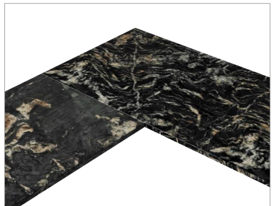
Example of a joint between two slabs, where the grain patterns do not "match" visually.
