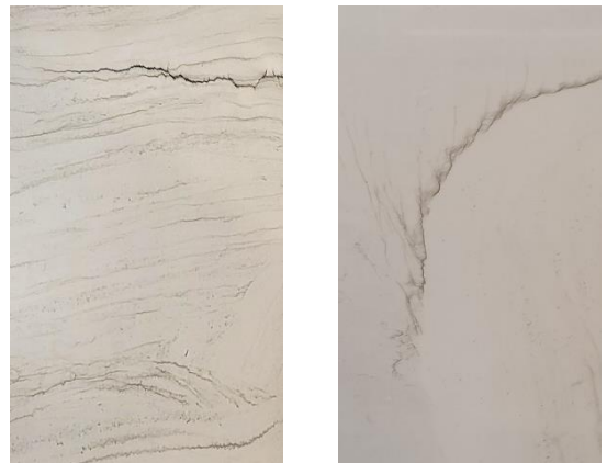
These images are two different slabs of the same type of stone. "Horizontal" pattern and "vertical" pattern
