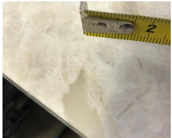
The mat monochrome spot is a resin surface-filler
