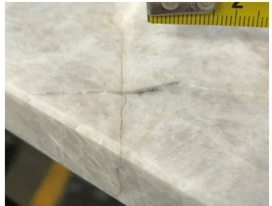
Here you can see a small glass vein which could be mistaken for a crack.
