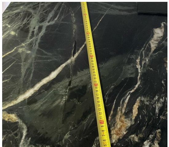
The matte black crack is a sparkle of a glass vein filled with dark resin.
