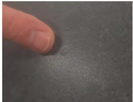
Example of an indentation that must be accepted
