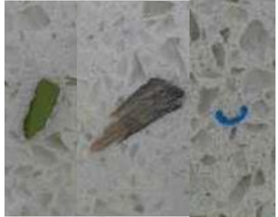
Here are examples of glass, wood and plastic that are not allowed in the surface
