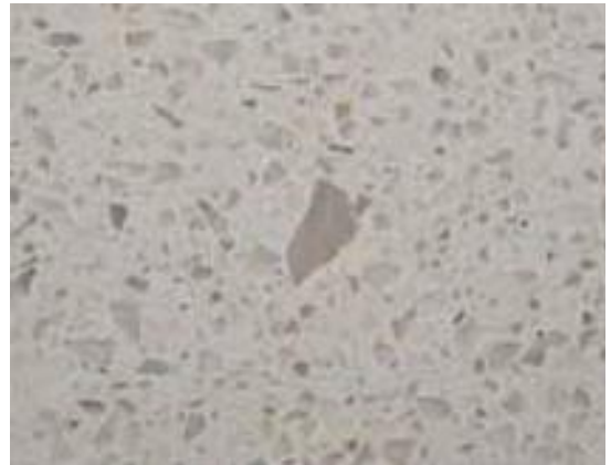
Example of quartz grains exceeding the maximum size
